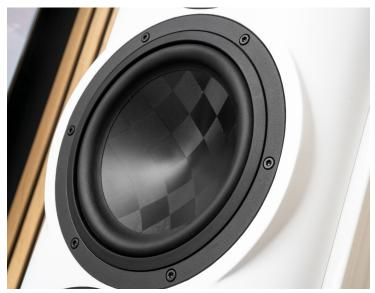
One of the two inner woofers. As with all four cone drivers, its cone is made of an extremely lightweight carbon fibre that is woven into a multi-layered yet thin-walled mesh. The lightweight and highly robust fabric enables high acoustic agility and impulse fidelity - and produces an attractive chequerboard look.
