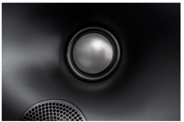
The main tweeter is positioned in the centre of the DPC array. It delivers the wide frequency range from 1.1 kilohertz to well over twenty kilohertz. This is made possible by the lightweight yet extremely hard beryllium membrane. The setback and the hornlike sound guide promote homogeneous interaction with the other drivers and the desired directional, wide dispersion
