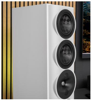
The shape of the attached baffle and especially the DPC array, which houses the three domes, ensures optimised sound dispersion in conjunction with the driver arrangement. With the cone woofers, there is a division of tasks: all four chassis start at around 20 hertz, the outer woofers then stop at 500 hertz, while the inner woofers work beyond that up to around 1.4 kilohertz. Here you can see the top partner of each woofer team.
