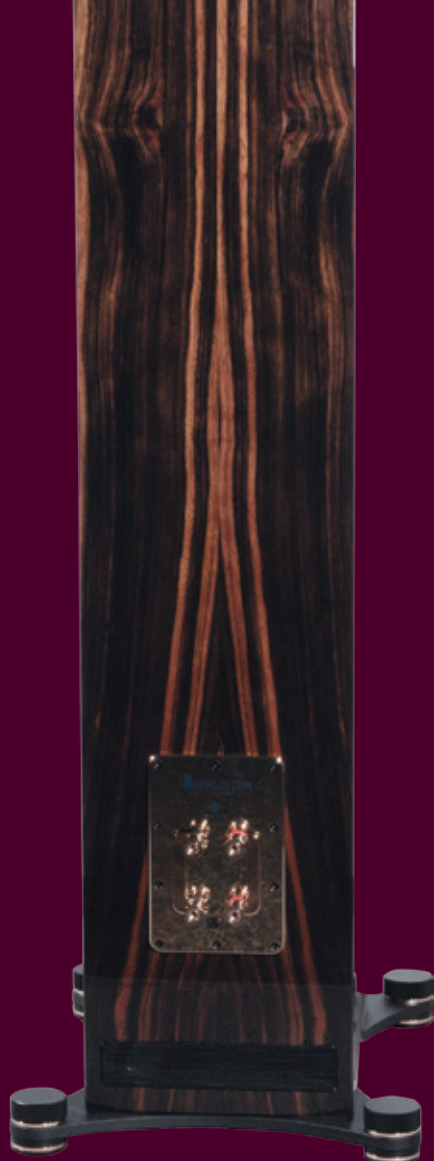
We find this grille in the bottom of the Perlisten, behind it is the bass reflex output – the S5t therefore work as a downfire
