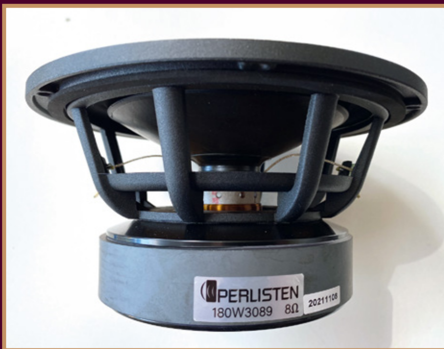
There are two of these 180 millimeter woofers in the Perlisten S5t. Its membrane consists of a Thin Ply Carbon Diaphragm - a very light carbon fiber
